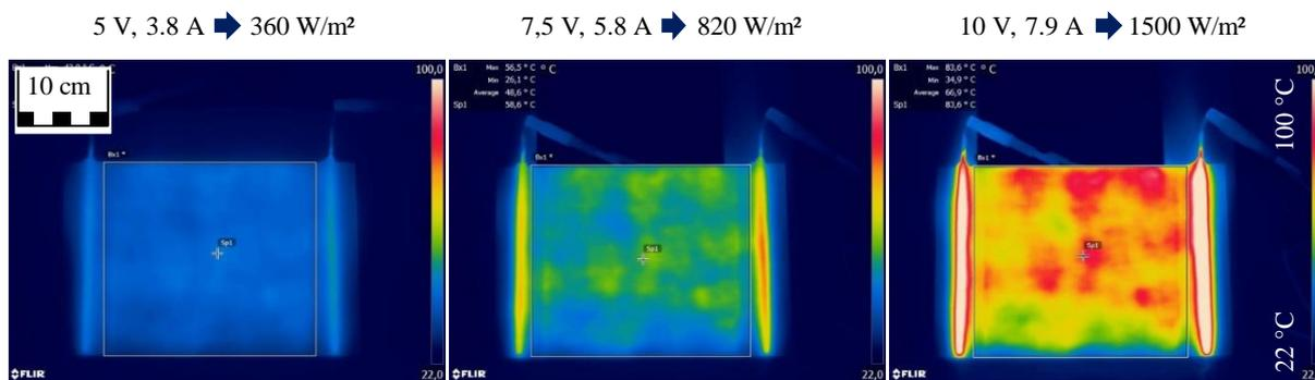
**Figure 1.** Sample plates of reinforced plastics from recycled carbon fibres as heating unit
