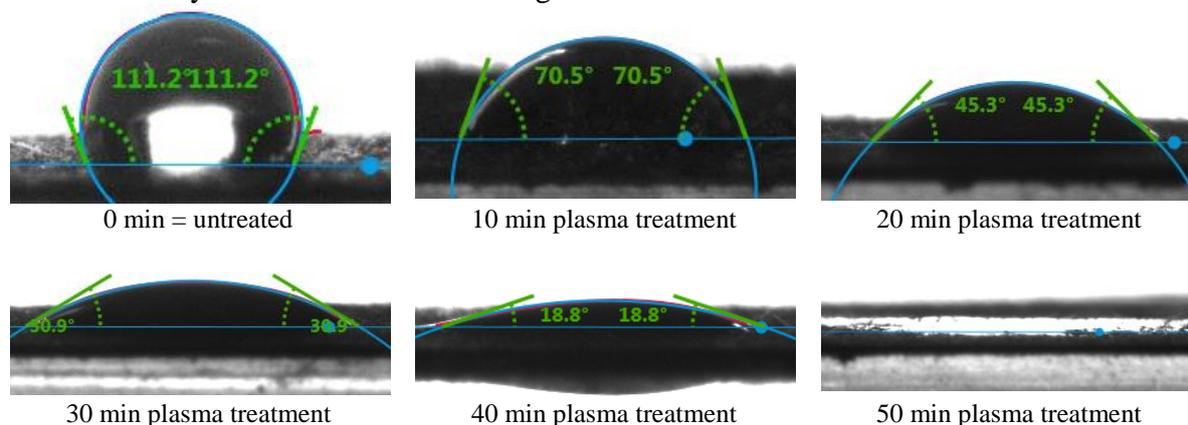
**Figure 1.** Examples of measurement of contact angle for evaluation of plasma treatment effect
