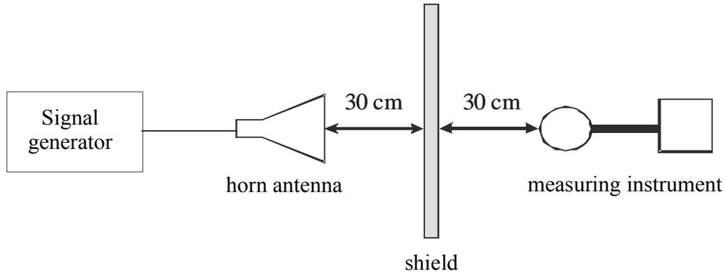
**Figure 1.** Measurement setup
