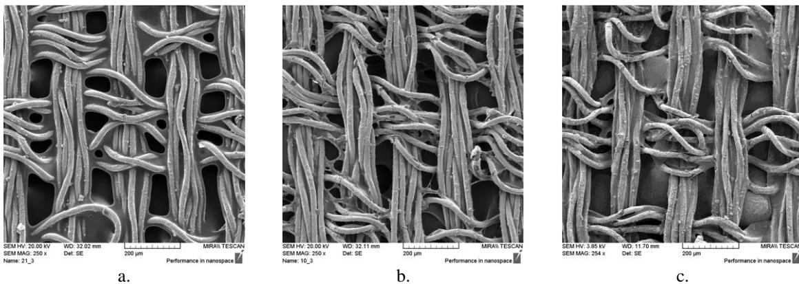
**Figure 2.** SEM images of polyamide fabrics metallized with copper: a. untreated; b. after 10 dry cleaning cycles; c. after 10 wet cleaning cycles
