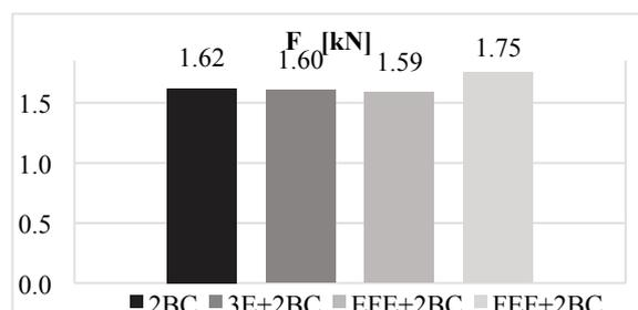
**Graph 2.** The force received under the anvil by the packages [kN]
