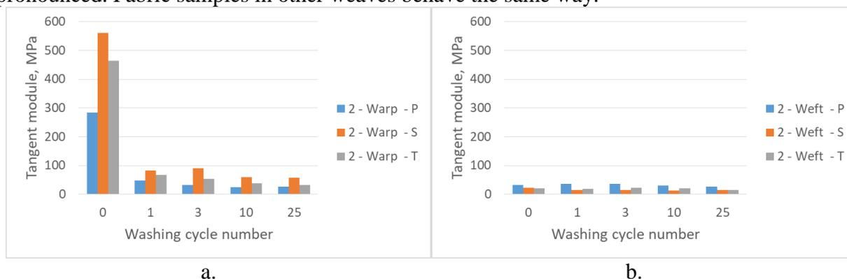
**Figure 2.** Tangent tensile module at 2% extension of the woven fabric samples, after 0, 1, 3, 10 and 25 washing cycles: a. warp direction, b. weft direction
