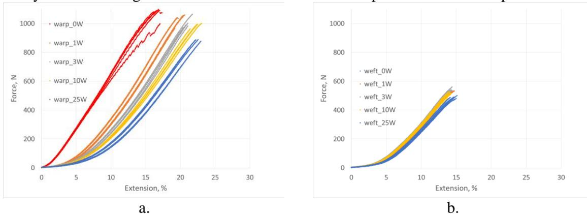
**Figure 1.** Tensile properties of the woven fabric sample, plain weave, after 0, 1, 3, 10 and 25 washing cycles: a. warp direction, b. weft direction
