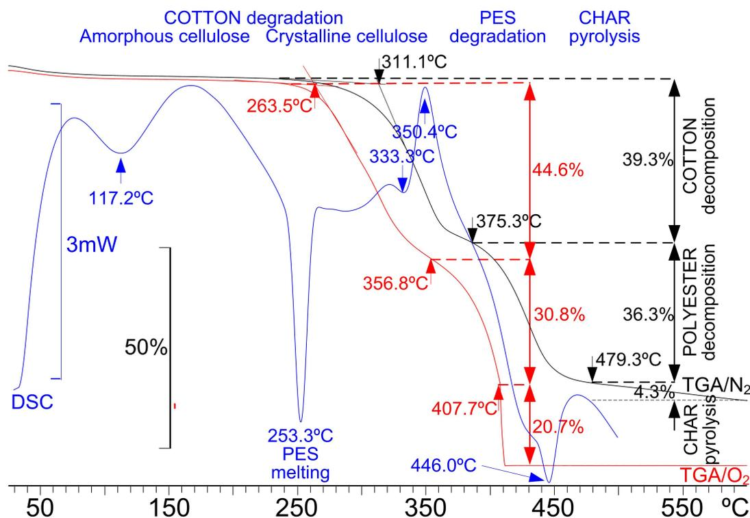
Figure 1: DSC and TGA plots in N<sub>2</sub> and O<sub>2</sub> atmospheres of the untreated mattress ticking of polyester/cotton plain weave of 177 g/m<sup>2</sup>.
