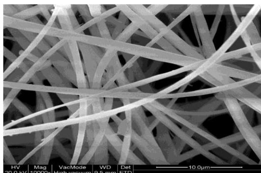
Figure 1. SEM images of electrospun silica nanofiber
