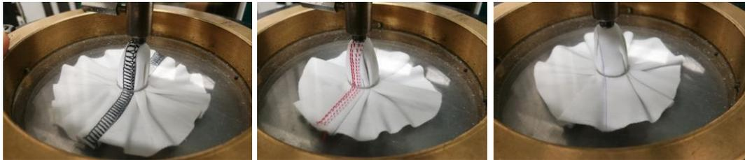
Figure 1. General views of hand test applying the device KTU-Griff-Tester
