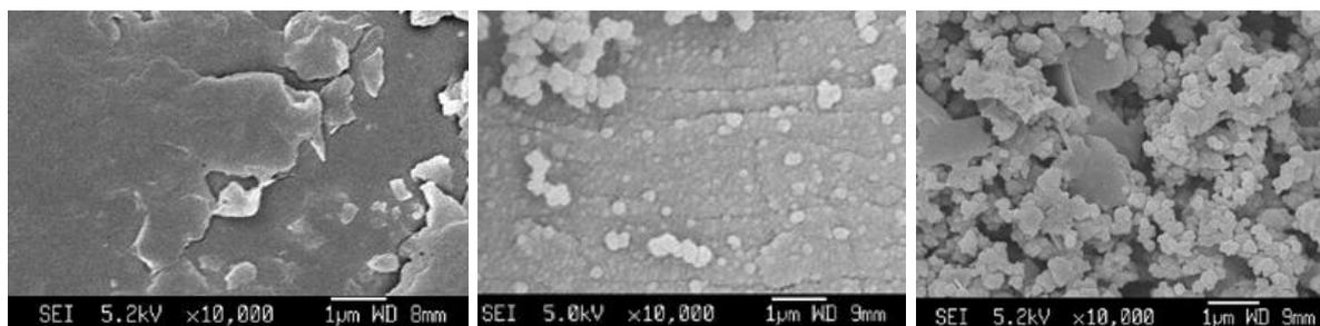
**Figure 3.** Initial membrane (top left), membrane coated with the application of iron chloride (top right) and with ammonium persulfate (bottom)
