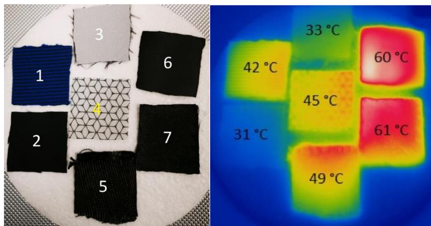
**Figure 4.** 1 – polyester/nylon 60/40 fabric with 20% graphene oxide; 2 – polyester lining fabric black colour; 3 – polyester shell fabric with white PU membrane; 4 – polyester fabric with 40% coverage print containing 18% graphene; 5 – pure carbon fiber fabric; 6 - polyester shell fabric with white PU membrane coated by polypyrrole; 7 – polyester fabric with PU membrane containing 18% of graphene oxide.
