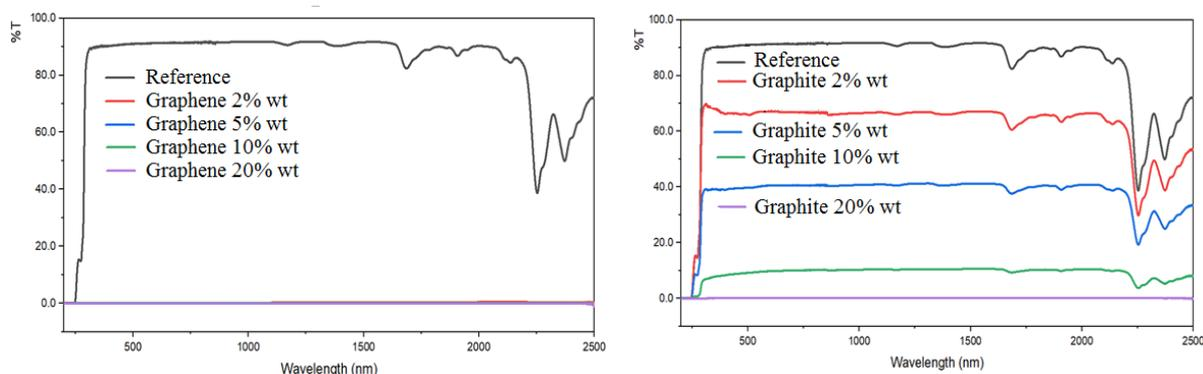
**Figure 1.** Heat transmittance of composites containing different amount of graphene and graphite
