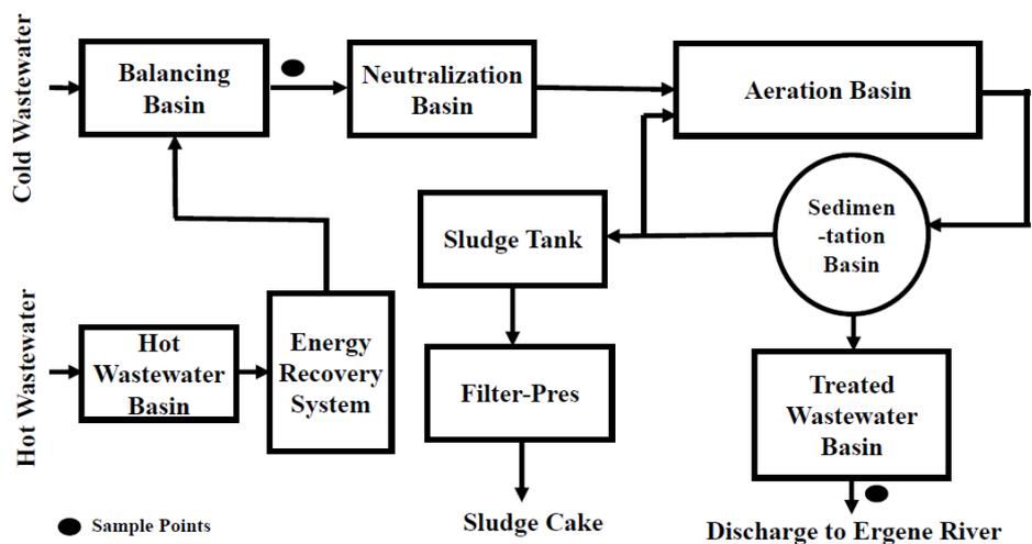
Figure 3. Flow diagram of investigated mill wastewater plant
