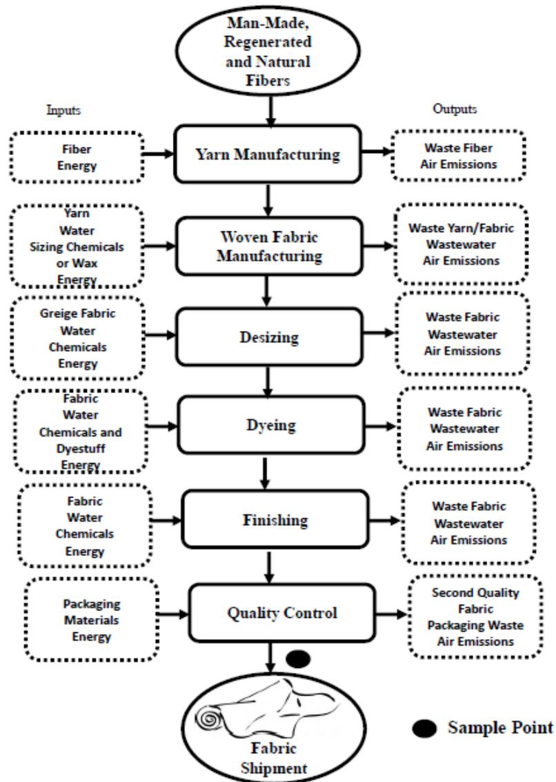
Figure 2. Flow diagram of investigated mill fabric production
