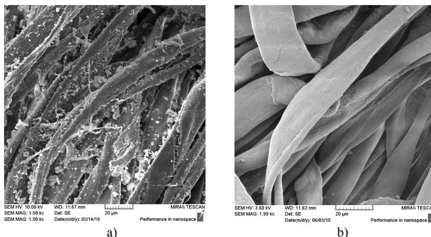
Figure 2. SEM micrographs of cotton fabric treated with Vibroactivated Zeolites –VZ\_5 (a) and Waterglass-WG10 (b)
