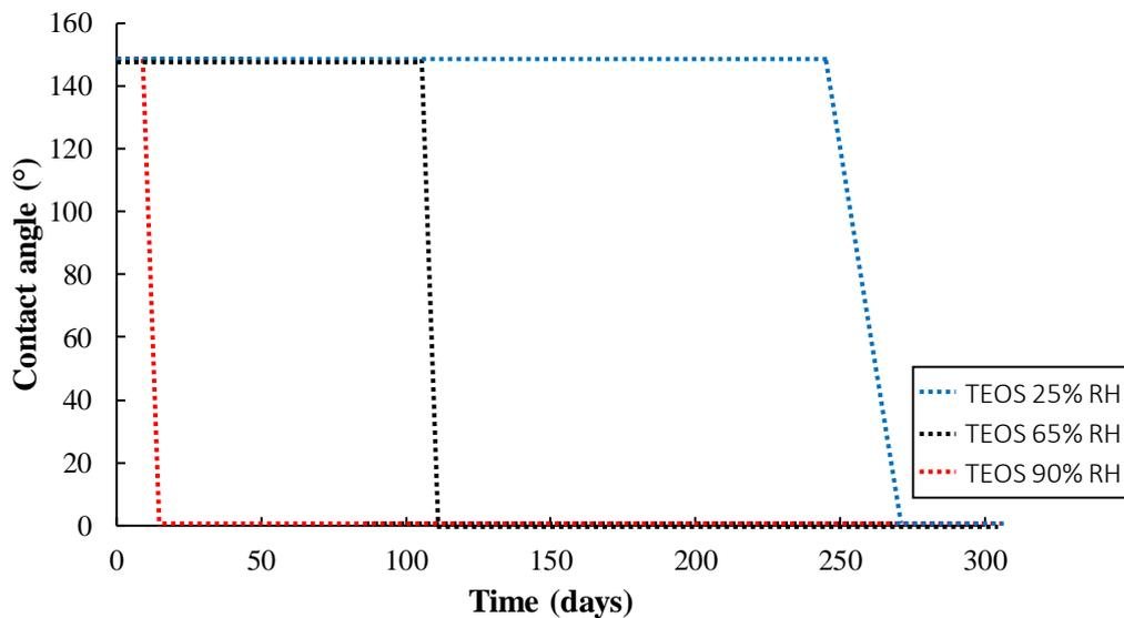
**Figure 4.** Water contact angle of silica nanofibers stored under controlled conditions of 20°C and 25, 65 and 90% RH. Just after the electrospinning the membrane is highly hydrophobic, with a contact angle around 150°.
