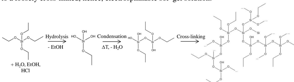
**Figure 1.** Principle of sol-gel synthesis for the direct electrospinning of silica nanofibers: the first step is an exothermal hydrolysis of the TEOS precursor, after which external heat allows for further condensation, resulting in a loosely cross-linked electrospinnable silica structure.
