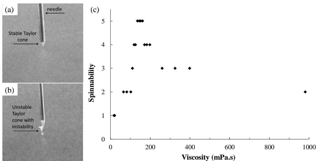
**Figure 2.** Electrospinnability of TEOS-based sol-gels by following the stability of the Taylor cone over time. Visualization of the Taylor cone: (a) Stable Taylor cone, (b) unstable, branched Taylor cone. (c) Electrospinnability as a function of the viscosity shows an optimal range between 120 and 200 mPa.s.
