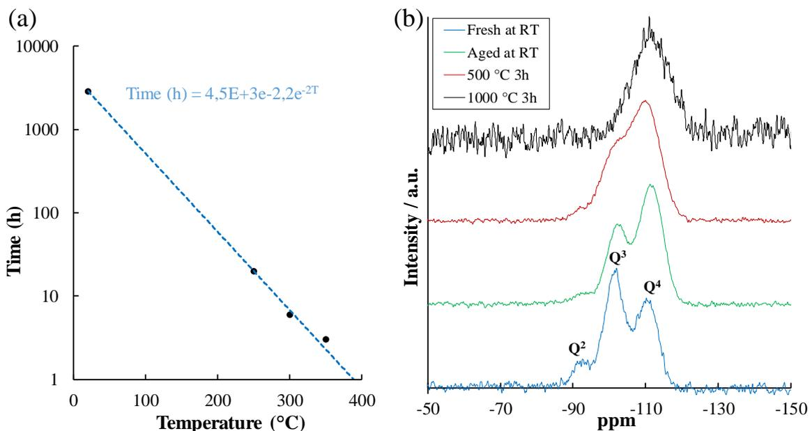
**Figure 5.** (a) Evolution of the heating time required for obtaining a superhydrophilic membrane as a function of the treatment temperature. The heating time increases exponentially upon lowering the heating temperature.
