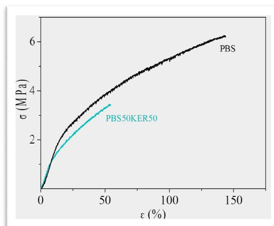
**Figure 2.** Stress-strain curves of the PBS and keratin/PBS 50/50 nanofibers
