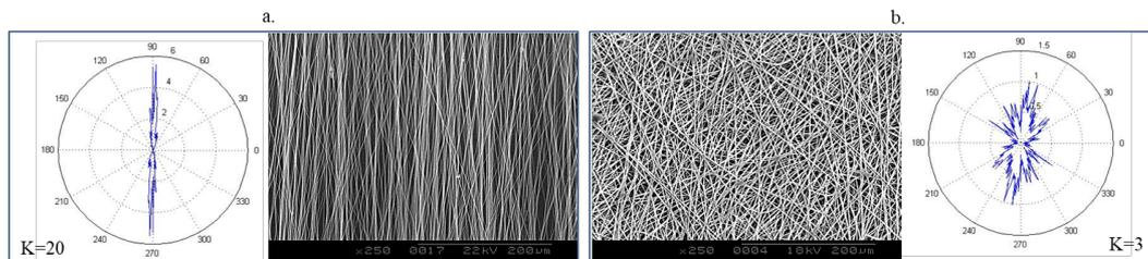
**Figure 1.** Different nano-filaments orientation histogram with given a numerical value of orientation (K)
