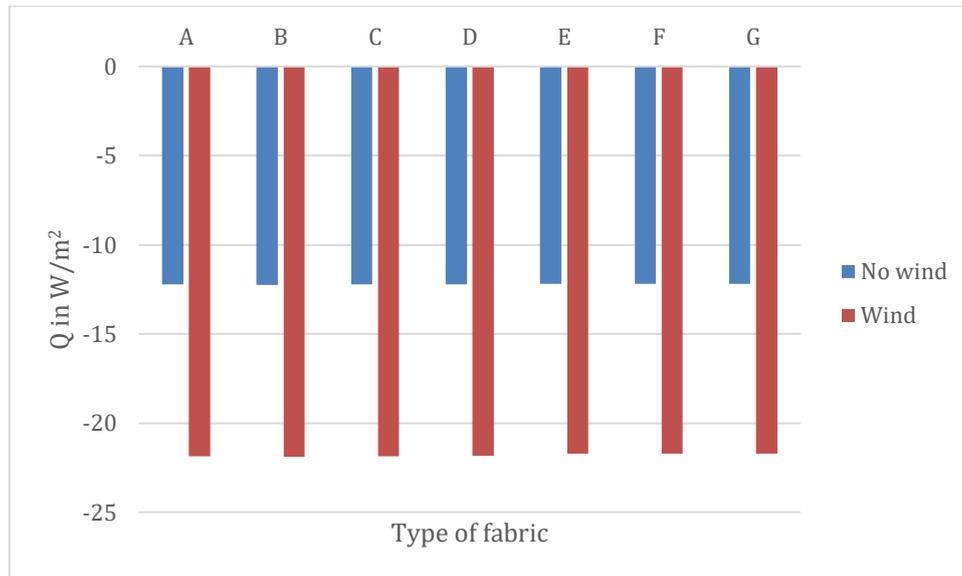
**Figure 2.** Heat transfer as a function of fabric type and wind.
