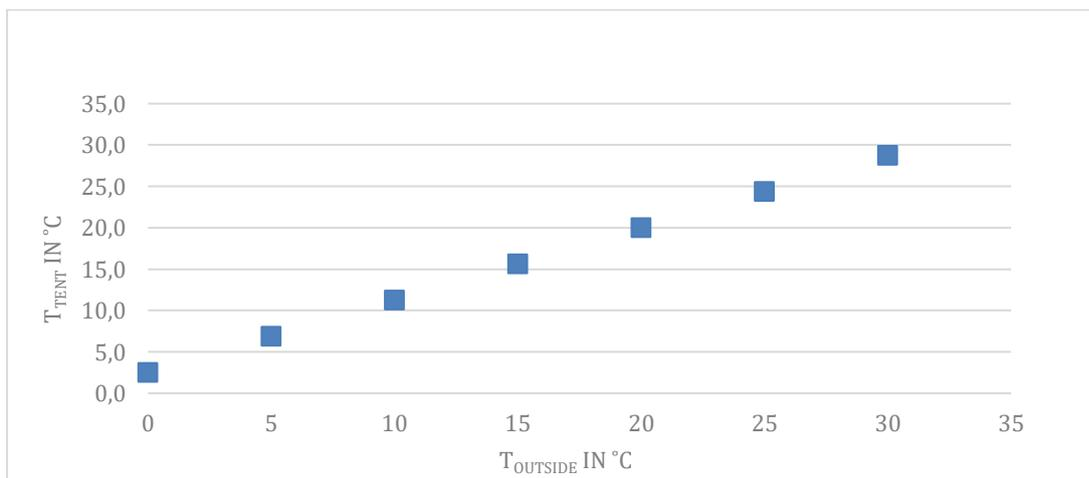
**Figure 4.** Temperature inner tent surface  $T_{tent}$  as a function of outside air temperature  $T_{outside}$
