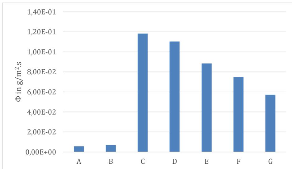
**Figure 3.** Water vapour transport as a function of fabric type.
