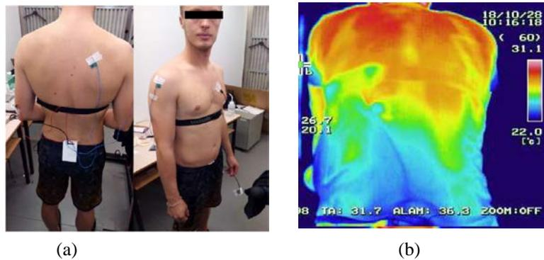
**Figure 4.** Receiver and sensors placed on the body (a) and thermal image of the back during the test (b)
