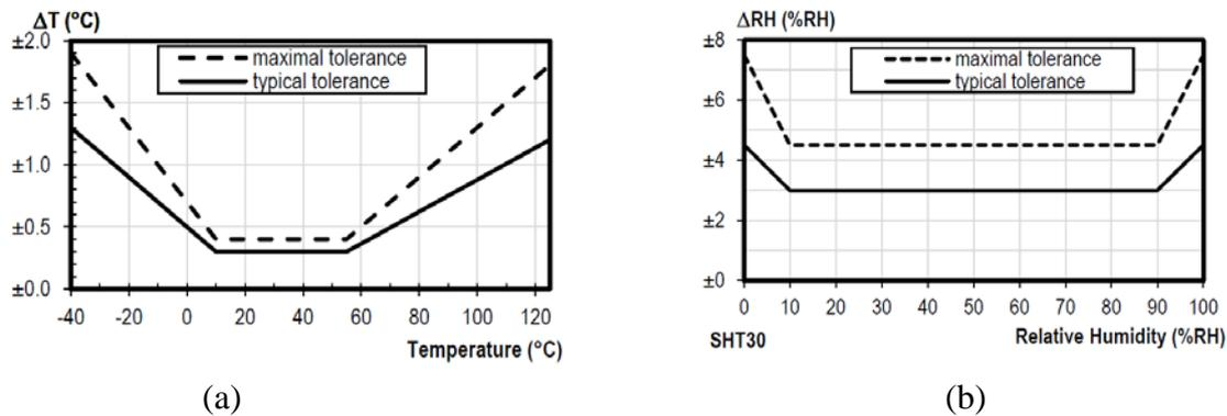
**Figure 2.** Tolerance of the temperature and humidity SHT31D sensor [SHT31D Datasheet]
