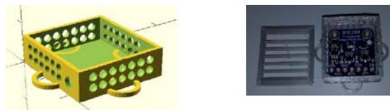
**Figure 3.** 3D-printed sensor holder.
