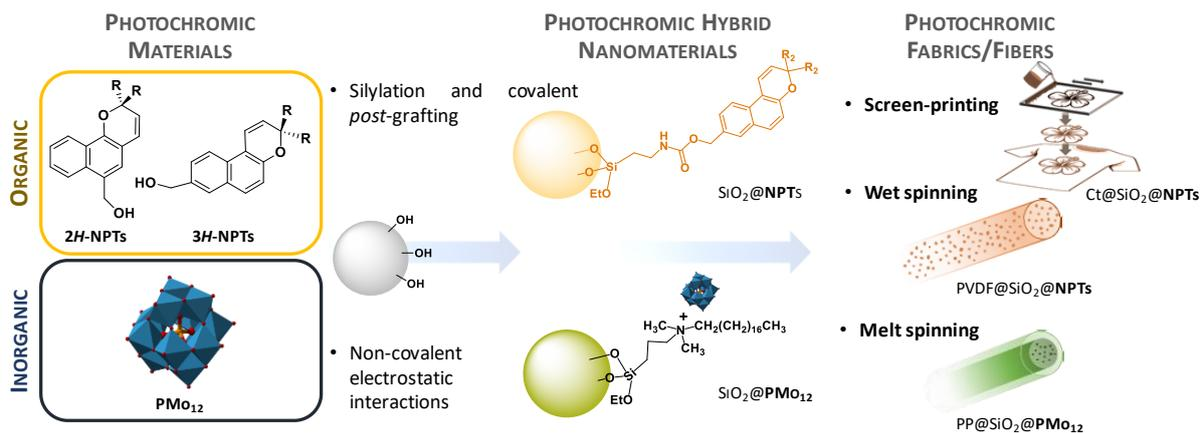
**Figure 1.** Schematic representation (not drawn to scale) of the immobilization of NPT derivatives (2H-NPTs and 3H-NPTs) and PMO<sub>12</sub> onto SiO<sub>2</sub> NPs and subsequent incorporation onto cotton fabrics by screen-printing or within PVDF and PP fibers by advanced fiber spinning technologies (wet spinning and melt spinning, respectively). Adapted with permission from refs. [23,27].
