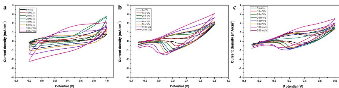
Figure 4. CV curves at varying potential scan rates ranging from 5 to 200  $\text{mV s}^{-1}$  (a) Pristine GO fiber, (b) Py/GO fiber, (c) PPy/GO fiber electrodes.
