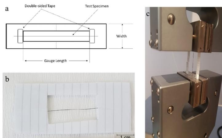
Figure 2. (a) Schematic of the test sample (b) Single fiber mechanical test sample (c) Implementation of single GO fiber for tensile testing.
