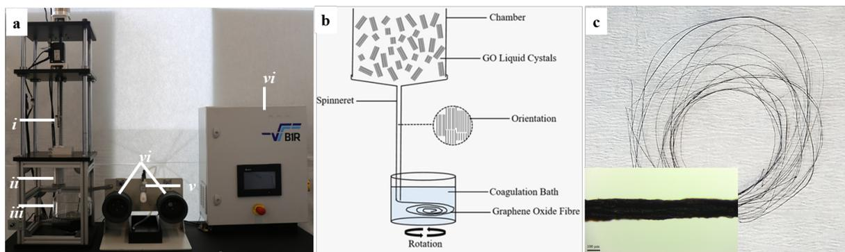
Figure 1. Custom-built GO wet spinning line at ITU ARC. a. (i) mixer and piston (ii) reservoir (iii) coagulation bath (iv) collecting drums (v) methanol shower (vi) control panel to adjust process parameters. b. Schematic view of drawing GO fibers and alignment of GO liquid crystals. c. True camera image and optical microscopy image of pristine GO fiber.
