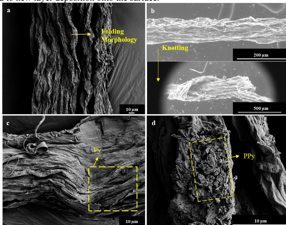
Figure 3. SEM images of the (a) knotting of pristine GO fiber (b) pristine GO fibers with folding morphology, (c) Py coated GO fibers, (d) PPy coated GO fibers.
