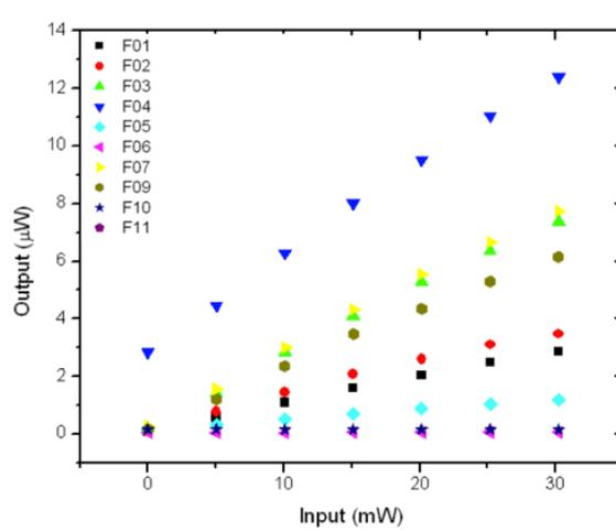
Figure 2 Measurements of the fibers light output at different incidenting light strenght for the evaluated fluorescent POFs (F01-F11).
