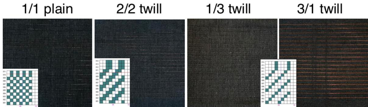
Figure 5: Woven smart patches using a dark brown Trevira CS yarn (256 picks/10 cm in warp direction and 297 ends /10 cm in weft direction).
