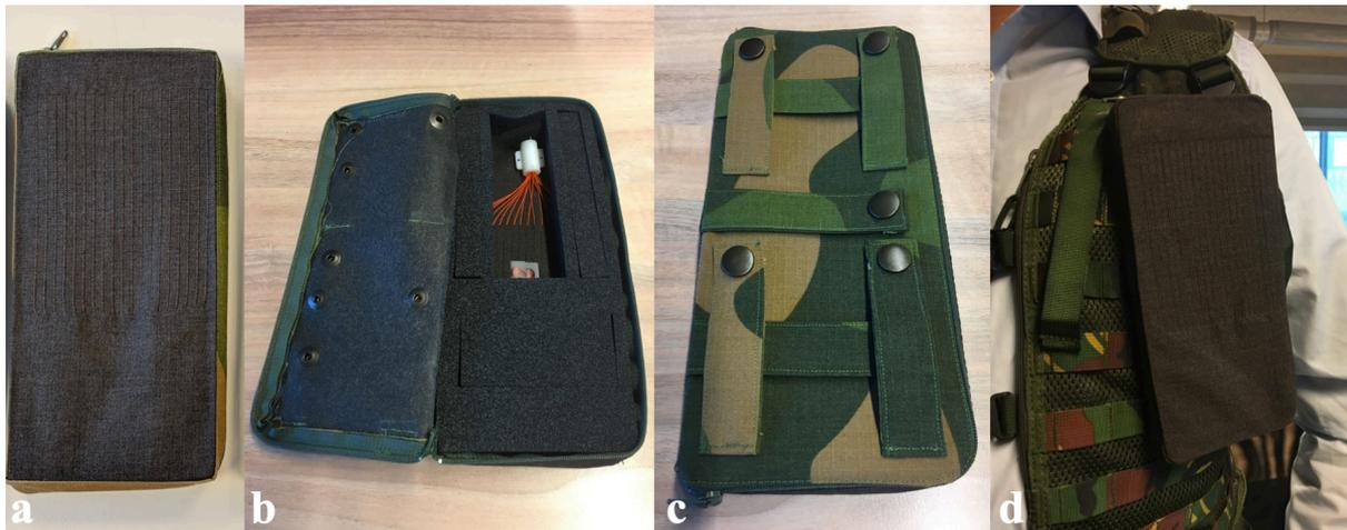
Figure 7 Smart patch with a 2/2 twill weave a) front view, b) open pouch w/o the read-out electronics, c) back view, d) smart patch attached to a combat vest.
