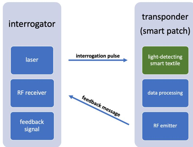
Figure 1 Schematic representation of the smart textile based remote identification system
