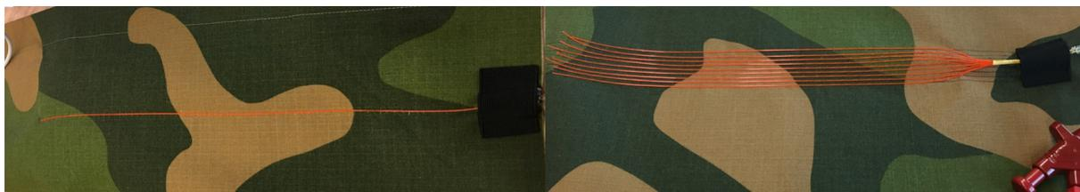
Figure 3 First prototypes of hand stitched optical fibers connected to a photodiode (1 vs 9 fibers).
