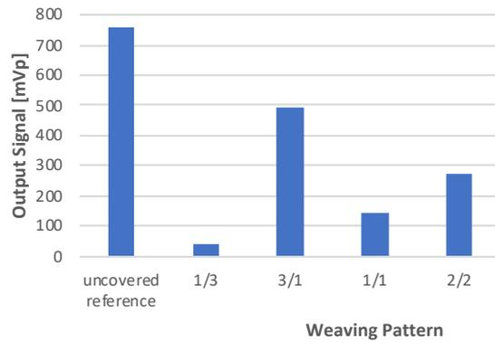
Figure 6 Impact of weaving pattern on output signal strength
