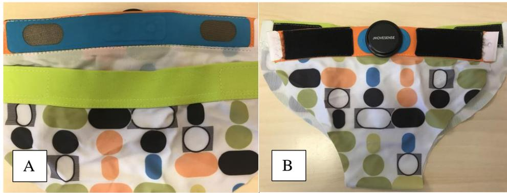
**Figure 2.** Mobile sleep pants with Movesense sensor and textile electrodes. A: skin side and B: the face side.
