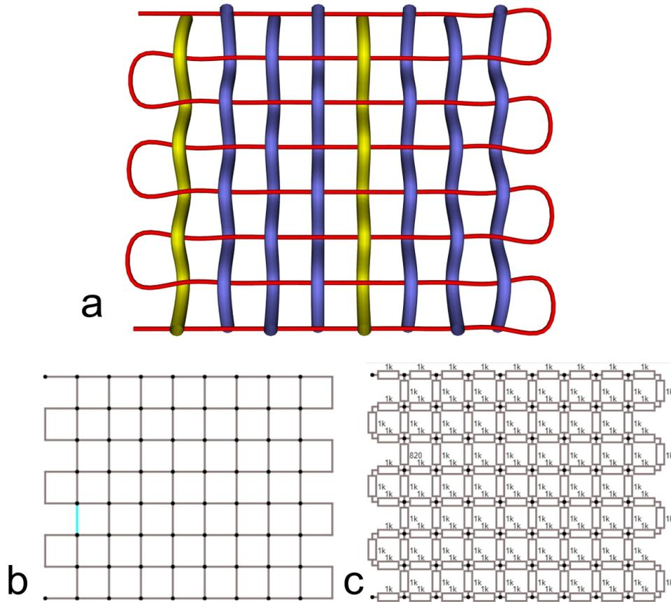
**Figure 4.** Simulated woven structure and its automatically generated circuits a) 3D geometrical model based on the TexMind Weaver b) circuit for the case of conductive yarns c) circuit for yarns with non negligible resistance
