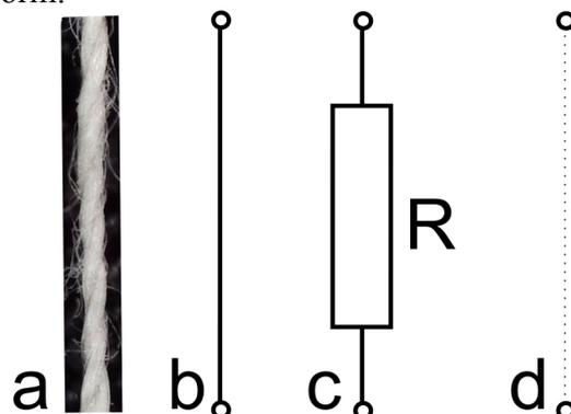
**Figure 1.** Textile yarn and its equivalents in the electric circuits a) staple fiber yarn b) representation as connecting wire without resistance c) representation as wire with some resistance d) isolator – the yarn does not need to be represented in the system
