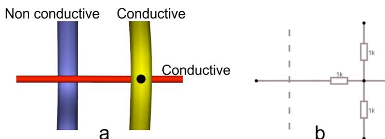
**Figure 2.** Crossing points between yarns with different electric conductivity. a) geometrical model b) equivalent circuit.
