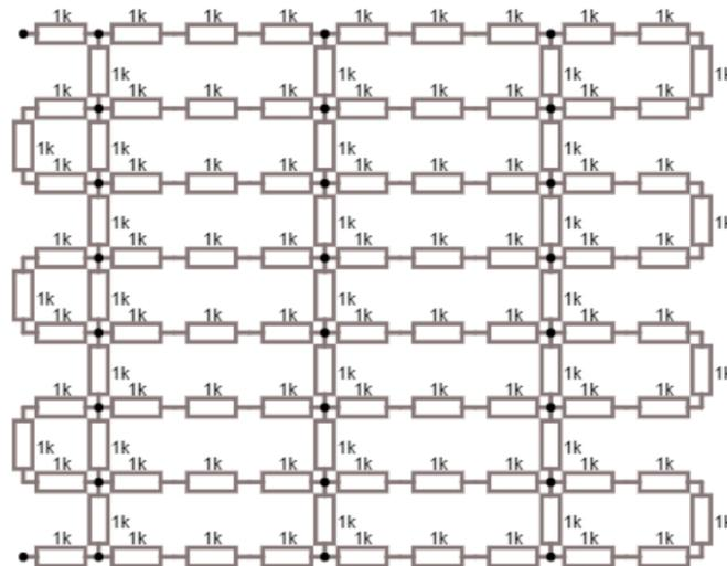
**Figure 5.** Circuit of the structure from Figure 4 for the case where after one conductive warp yarn two non-conductive warp yarns are placed.
