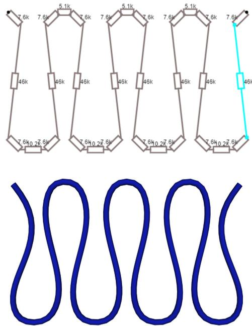
**Figure 6.** 3D Model of one row of weft knitted structure and its equivalent electric circuit
