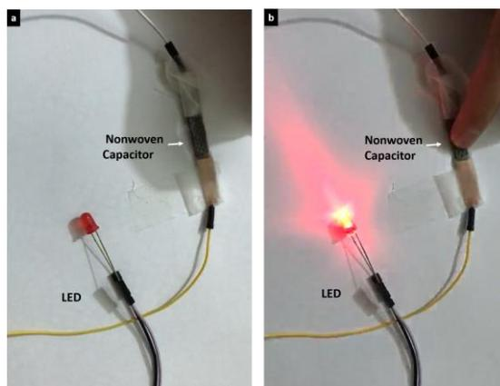
**Figure 6.** Conductive nonwoven sample was used as a capacitive sensor to light up an LED.
