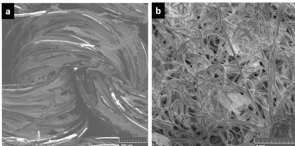
**Figure 2.** SEM image of AgNW coated knitted fabric (a) and nonwoven sample (b). Scale bars are given on the lower right corner of the images.
