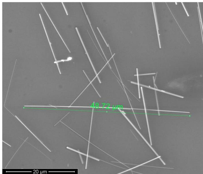
**Figure 1.** SEM image of AgNWs under 5000 magnifications. Scale bar is given on the lower left corner of the image.
