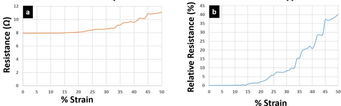
**Figure 5.** (a) Resistance versus % strain plot (a) and % increase in resistance versus % strain plot for conductive knitted sample. Distance between the two gauges was 3.5 cm. Thus, initial resistance of the sample was 2.3 Ω/cm.
