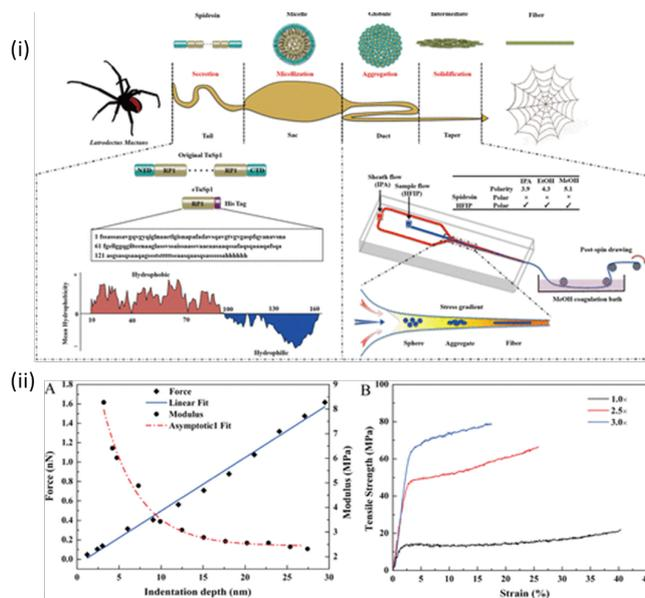
Fig. 6 (i) Schematic of the silk fiber assembly by a biomimetic microfluidic device. A spider's gland, consisting of a tail, sac, duct, and taper, is illustrated with corresponding function of protein secretion, micellization, induced aggregation and
