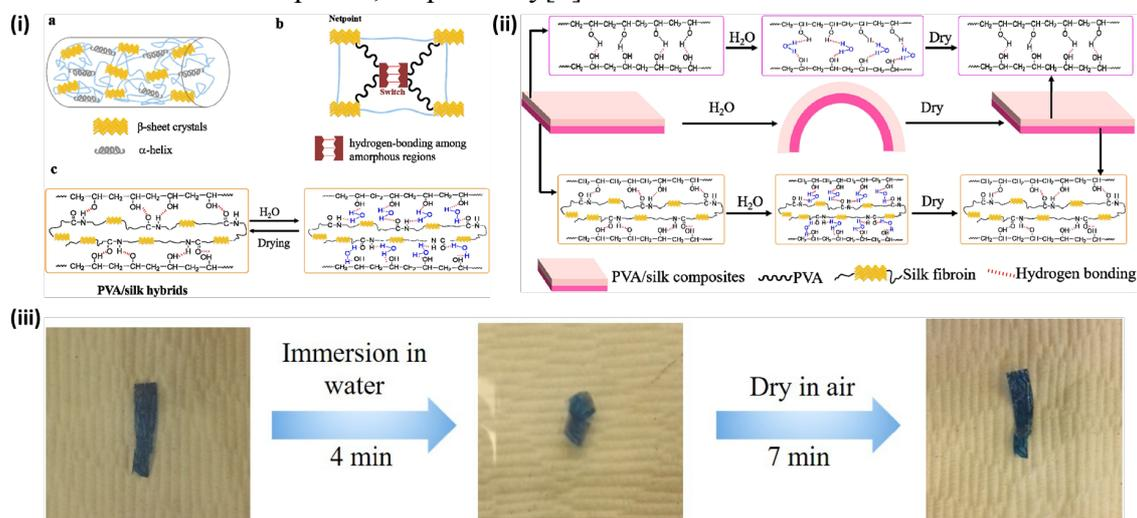
Fig. 3 (i) (a) Structural model of silk (spider silk, silkworm silk) and (b) proposed water-sensitive shape memory mechanical model of spider silk. (c) Cleavage and reforming of hydrogen bonds between PVA and silk under effect of water (ii) Schematic illustration of the two-way shape-memory behavior of PVA/silk hybrids actuated with water (iii) Photography showing water-sensitive two-way shape-memory effect of PVA/10% silk hybrid
