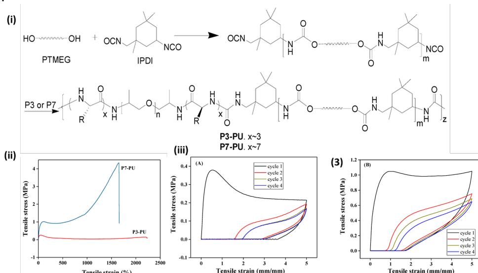
Fig. 2 (i) Synthesis of the obtained peptide-polyurethane/ureas (P3-PU and P7-PU) (ii) Stress-strain curves of (P3-PU and P7-PU) (iii) Cyclic Tensile curves of P3-PU(A) and P7-PU(B) at 500% strain
