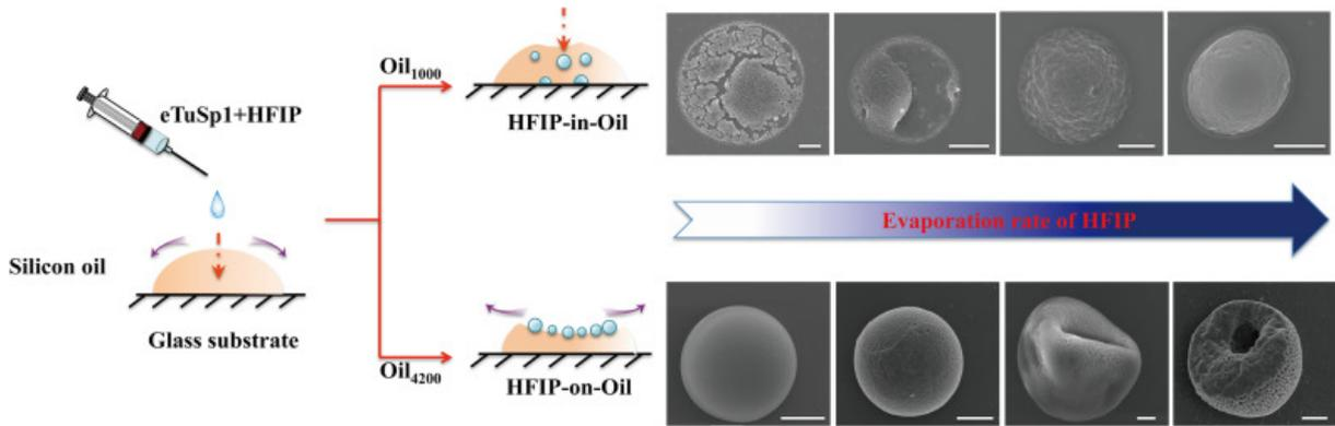
Fig. 4 Fabrication of spider silk spheres in an HFIP-Oil system. Oil<sub>1000</sub>: silicon oil with  $M_w$  of 1000; Oil<sub>4200</sub>: silicon oil with  $M_w$  of 4200. Scale bar is 10  $\mu\text{m}$ . Accompanied by evaporation of HFIP, various silk morphologies could be observed in two different modes.
