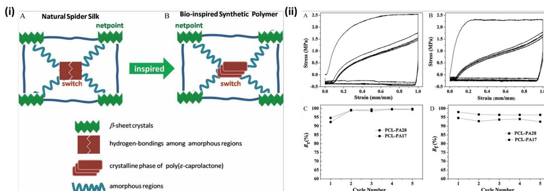
Fig. 1 (i) Shape-memory structural models of: A) natural spider silks and B) bioinspired synthetic polymers. (ii) Shape-memory properties of bioinspired copolymers. A,B) Typical cyclic tensile tests for PCL-PA17 and PCL-PA28, respectively. C) Shape recovery ratio ( $R_r$ ) and D) shape fixing ratio ( $R_f$ ) for five cycles when  $e_m \frac{1}{4} 100\%$
