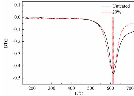
**Figure 3.** DTG curves of PI fibers
