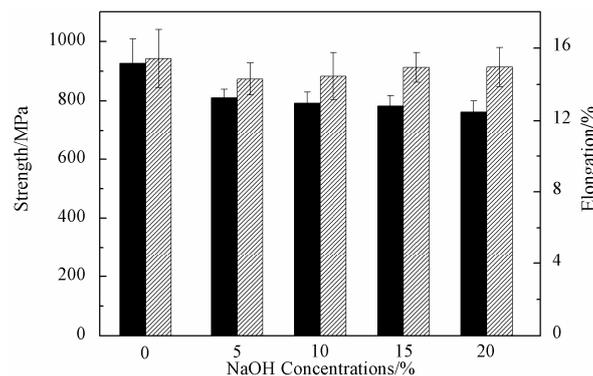
**Figure 1.** Tensile strength and elongation of PI fiber by NaOH treatment
