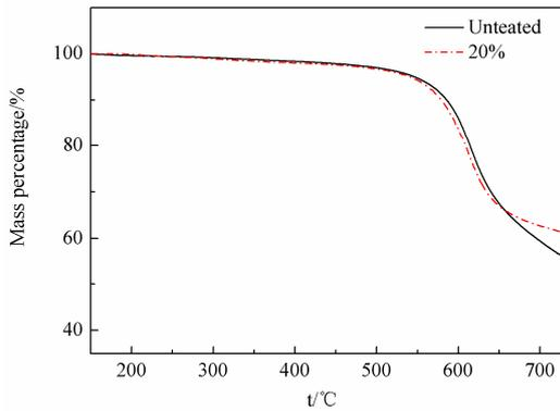
**Figure 2.** TGA curves of PI fibers
