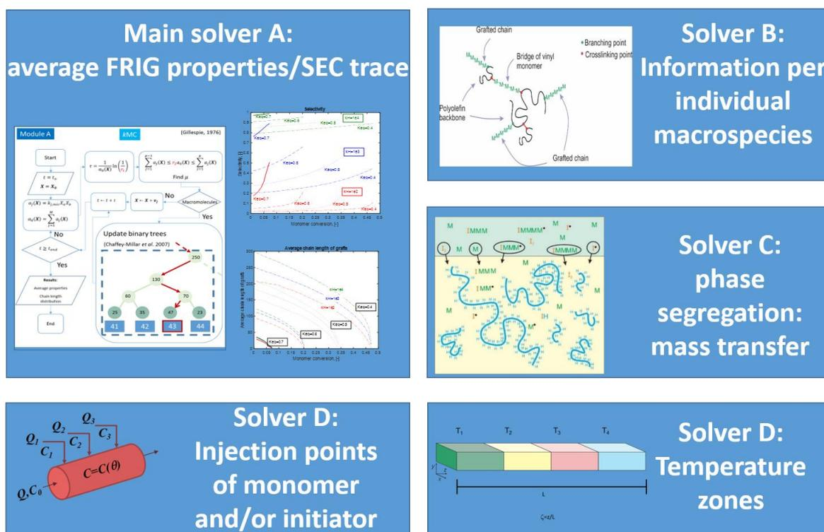
**Figure 1.** Workflow regarding modeling platform to describe FRIG kinetics under single and multiphase reaction conditions; the former can be mimicked by long mixing times; the latter result under time scale typical for reactive processing at industrial scale.
