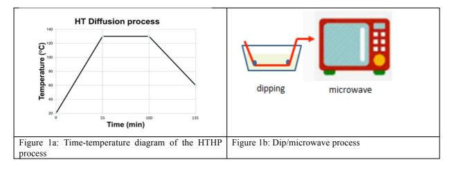
The temperature of the exhaustion bath was gradually raised (about 2°C/min) to 130°C, and was kept at this temperature for about 45 min. The bath was then cooled to 60°C; then the
