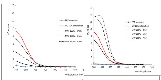
Figure 3a: Spectral curves of polyester fabric with vanillin solution subjected to microwaves at  $125~\mathrm{W}$
