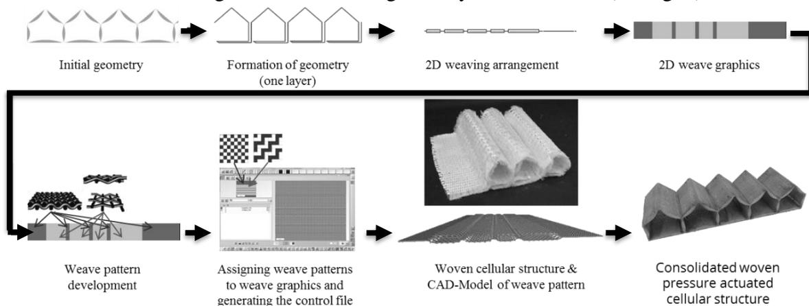
Fig. 1: Process chain for the woven cellular structures
