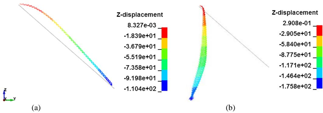
Figure 4. Simulation of cantilever test of textile: (a) correct bending rigidity (b) lower bending rigidity
