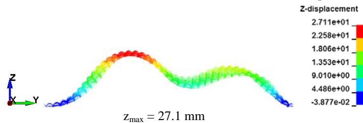
Figure 6. Compressive deformation of textile models with lower bending rigidity
