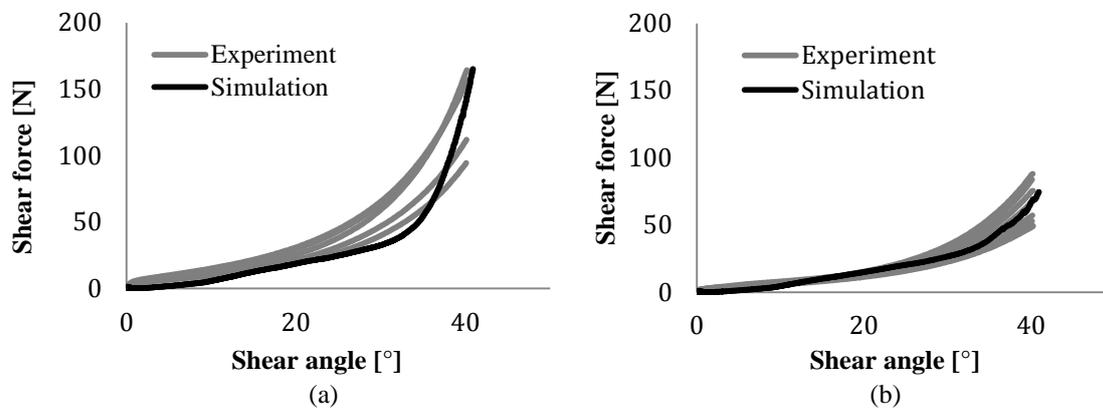
**Figure 9.** Comparison of shear force – shear angle curve between simulation and experiment of (a) Variant 1 and (b) Variant 2
