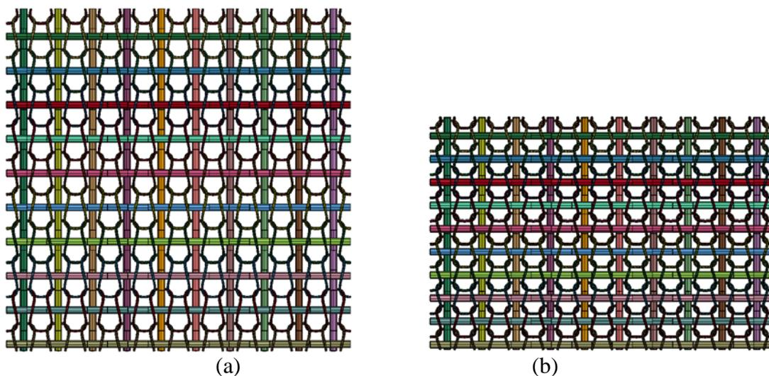
**Figure 3.** Comparison of the meso-scale models of the two fabric variants: (a) Variant 1 (b) Variant 2
