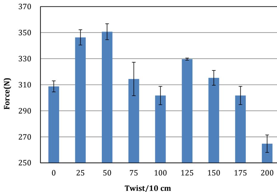
**Figure 1.** The breaking forces of different twists yarns
