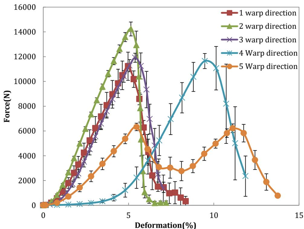
Figure 2. Warp direction tensile tests results of five structures
