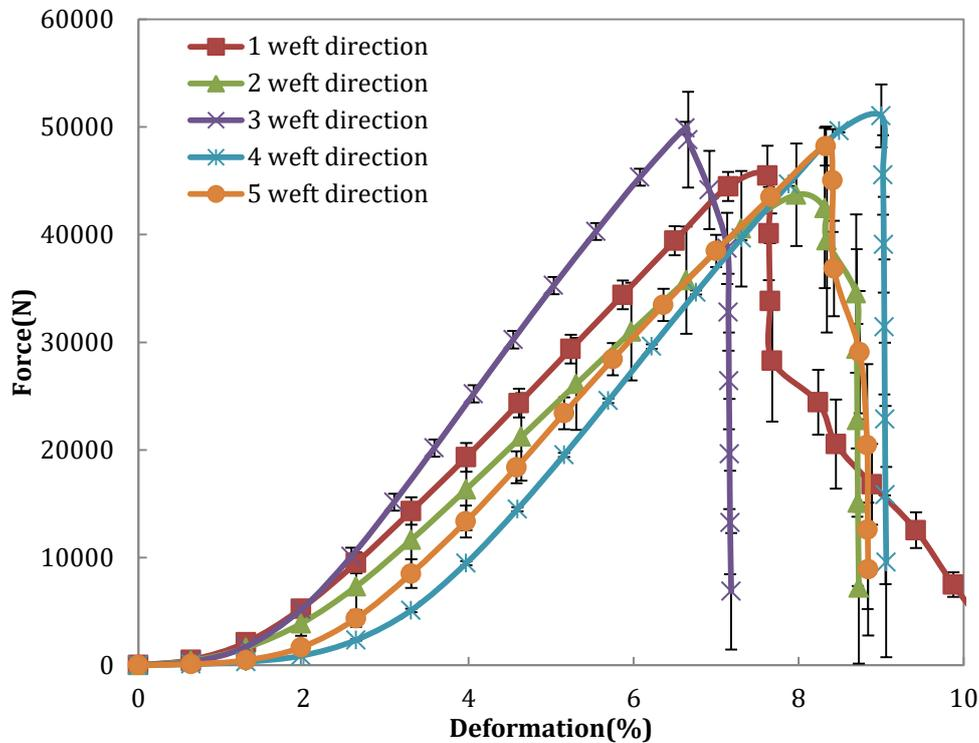
Figure 3. Weft direction tensile tests results of five structures.
