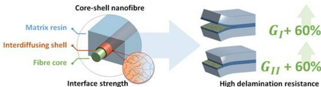
**Figure 3.** Concept of interdiffusing core-shell structured coaxial nanofibres. The (polycaprolactone) shell will dissolve/diffuse into the matrix resin forming a strong bond between the matrix resin and the nanofibre cores. This leads to a simultaneous increase in Mode I and Mode II delamination resistance.
