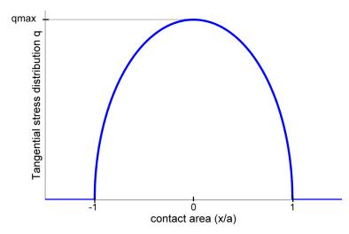
Figure 5. Tangential stress distribution q in a line contact with  $F_N > 0$ ;  $Q > \mu F_N 0$ ;  $F_{fat} = 0$ .
