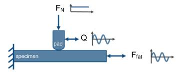
Figure 1. Overview of interacting forces  $F_N$ , Q &  $F_{tat}$  on fretting fatigue contact between pad and specimen.
