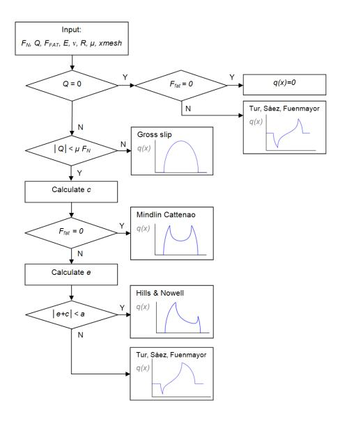
Figure 10. Flowchart to calculate tangential stress q(x).
