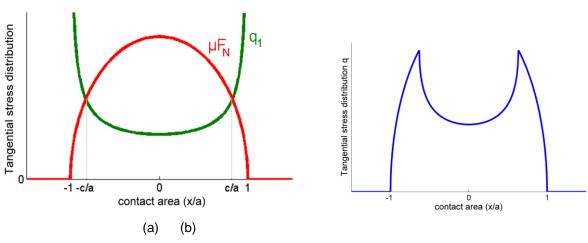
Figure 6. Tangential stress distribution q in a line contact with  $F_N > 0$ ;  $Q \neq 0$ ;  $F_{fat} = 0$ .
