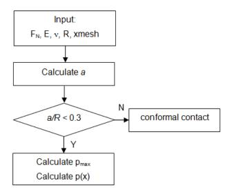
Figure 4. Flow chart to calculate normal stress distribution (Hertz) in Matlab.
