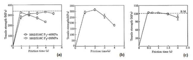
Fig. 4: Tensile strength vs. friction time for friction welds of steel S10C to aluminium alloys A5052 (a), A5083 (b) and A1070 (c). P<sub>1</sub> resembles the friction pressure during the friction phase.
