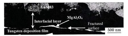
Fig. 7: Fractured surface observed in a joint bonded at friction time of 4 s
