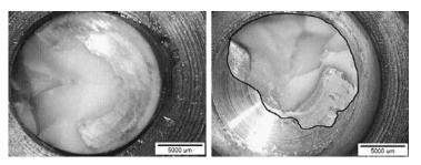
Fig. 11: Pictures of bonds destroyed during tensile tests.
