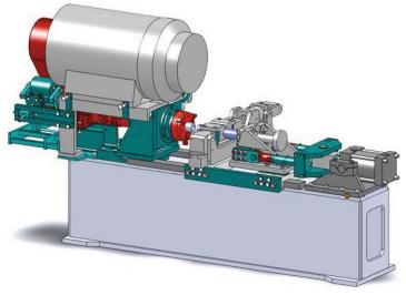
Fig. 2: Redesign of the rotary friction welding machine (2)
