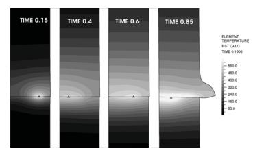
Fig. 9: Temperature distributions in the welded materials for selected values of friction time.
