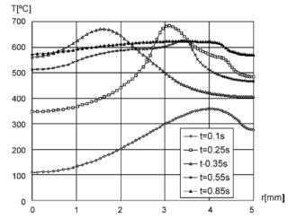
Fig. 8: Temperature variation over the joint interface for selected values of heating time.
