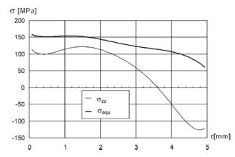
Fig. 13: Residual stress profile in a ceramic workpiece near the bond area obtained by FEM.
