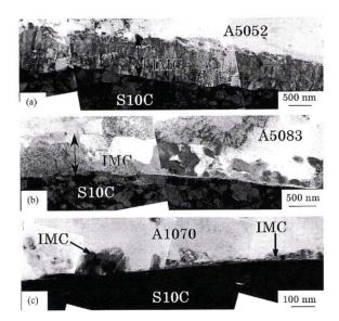
Fig. 6: IMC layers observed at friction-bonded interfaces: (a)A5052/S10C joint ( $P_1$ =40MPa,  $t_1$ =4s), (b) A5083/S10C joint ( $P_1$ =40MPa,  $t_1$ =3s), and (c) A1070/S10C joint ( $P_1$ =20MPa,  $t_1$ =2s).  $t_1$  resembles the duration of the friction phase.
