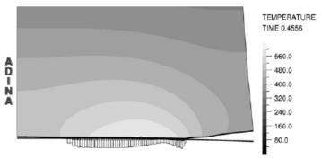
Fig. 10: Deformation of AI in the vicinity of the contact zone scaled up eight times, bands of equal temperature and contact force distribution (time of heating 0.455 s)
