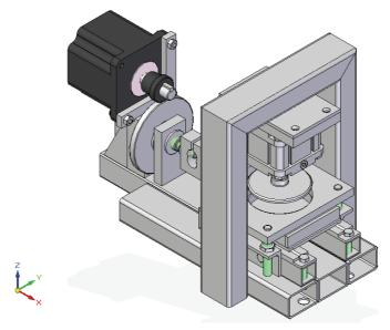
Figure 3. Automatic shear testing device
