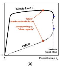
Figure 4. The analysis of a result with net section collapse is more intuitive in terms of remote strain:
