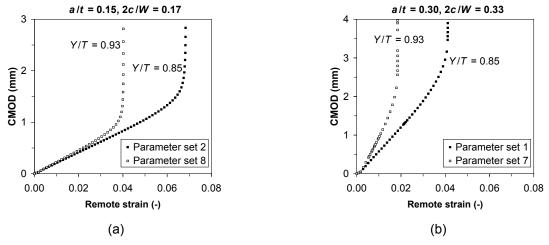
Figure 8. Y/T has a pronounced influence on strain capacity. As regards the CMOD response prior to net section collapse, its influence is significant for large defects (b), but marginal for small defects (a).
