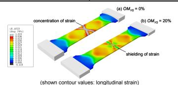
Figure 6. A weld which is overmatched in strength (b – parameter set 11) shields the weld defect from applied deformations, which is not the case for an evenly matching weld (a – parameter set 1).
