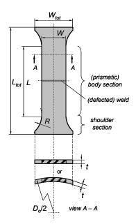
Figure 1. Configuration of a mini wide plate tension test.
