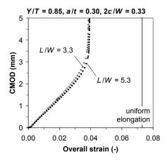
Figure 13. Both specimen designs result in a similar CMOD response.
