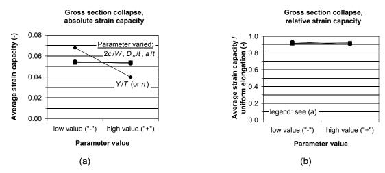
Figure 11. Averagely obtained (a) strain capacities and (b) relative strain capacities, for the simulations with gross section collapse ( $OM_{YS} = 20\%$ ).
