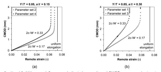
Figure 9. a/t and 2c/W have an influence on both strain capacity and CMOD response prior to net section collapse. The influence of 2c/W is more pronounced for higher a/t-values (b) than for lower a/t-values (a).
