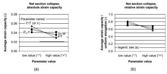
Figure 7. Averagely obtained (a) strain capacities and (b) relative strain capacities, for the simulations with net section collapse ( $OM_{YS} = 0\%$ ).
