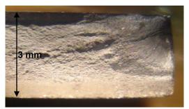
Figure 17. Fracture surface of specimen at stress of 110 MPa and 350°c
