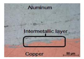
Figure 5: Microscopic image of a copper-aluminium MPW weld
