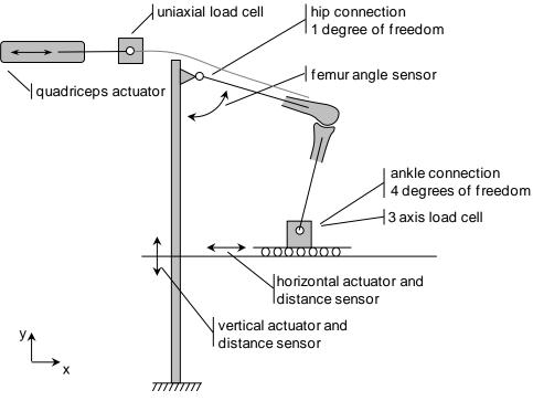
Figure 2: Schematic representation of the knee rig.
