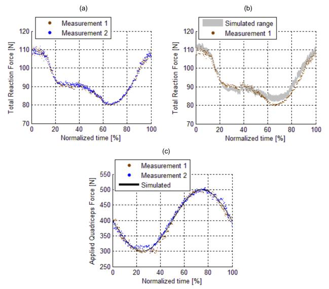
Figure 6: Modelling and measuring of the hinge model at the UGent Knee Simulator. a) The total ankle reaction force of the two measurements, b) Measurement 1 of the ankle force compared with the simulated surface ,c) The applied quadriceps force of the measurements.
