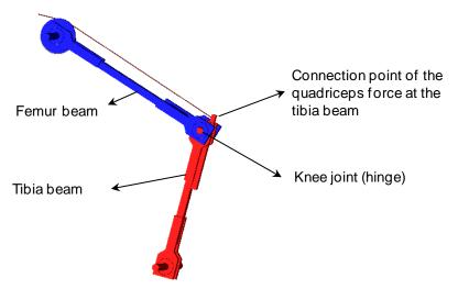
Figure 3: Schematic representation of the mechanical hinge model.
