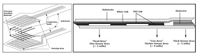
Figure 1: Construction Tekscan sensor [7]
